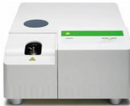
Differential scanning calorimetry (DSC822e, Mettler Toledo, USA). Test the heat of fusion of phase change materials (PCMs)
