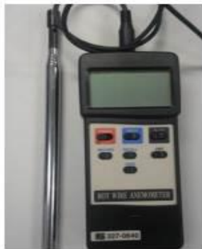
Hot wire anemometer (RS327-0640, Tecpel, Taiwan). Measure the air velocity of the ventilation fans
