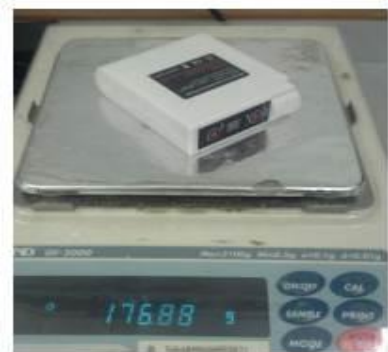
Electronic balance (GF-2000, A&D, Japan). Measure the weight of the cooling sources
